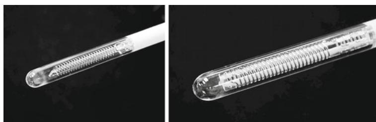
**Fig. 2** Sensors with strip support and cross support
