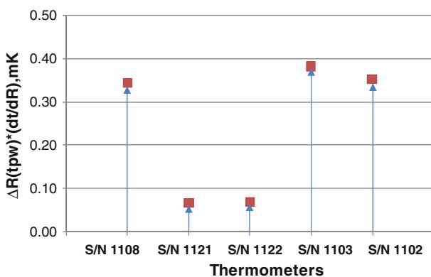
**Fig. 7**  $R$  (tpw) changes after five thermal cycles from room temperature to 1085 °C
