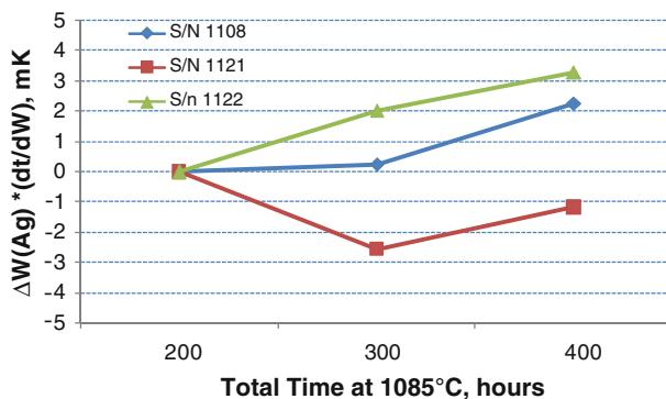
**Fig. 4** Long-term stability at the freezing point of silver
